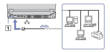
If the main unit is docked, you can only use the ethernet network connector on the docking station.
